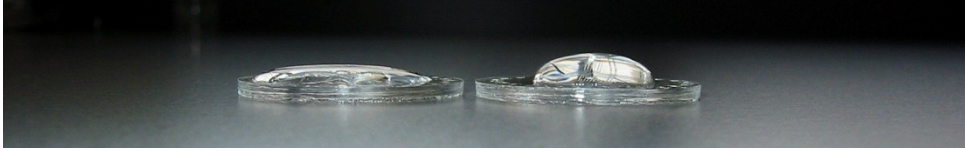
Fig. 3.9. The increased hydrophilicity of PDMS after coating with PEG visualized by the decreased contact angle of the water droplet on top of the PDMS on the left, and the untreated hydrophobic PDMS on the right.
